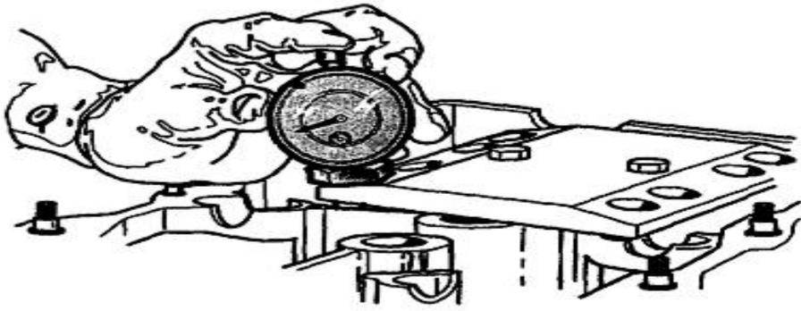
This is a factory Nissan tool to measure valve tip height!
